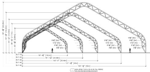
Supa-Span T profile is designed with a triangular curved high pitched roof and eave assembly ranging from 18m - 50m standard span. Larger spans can be engineered to meet your exact needs.
